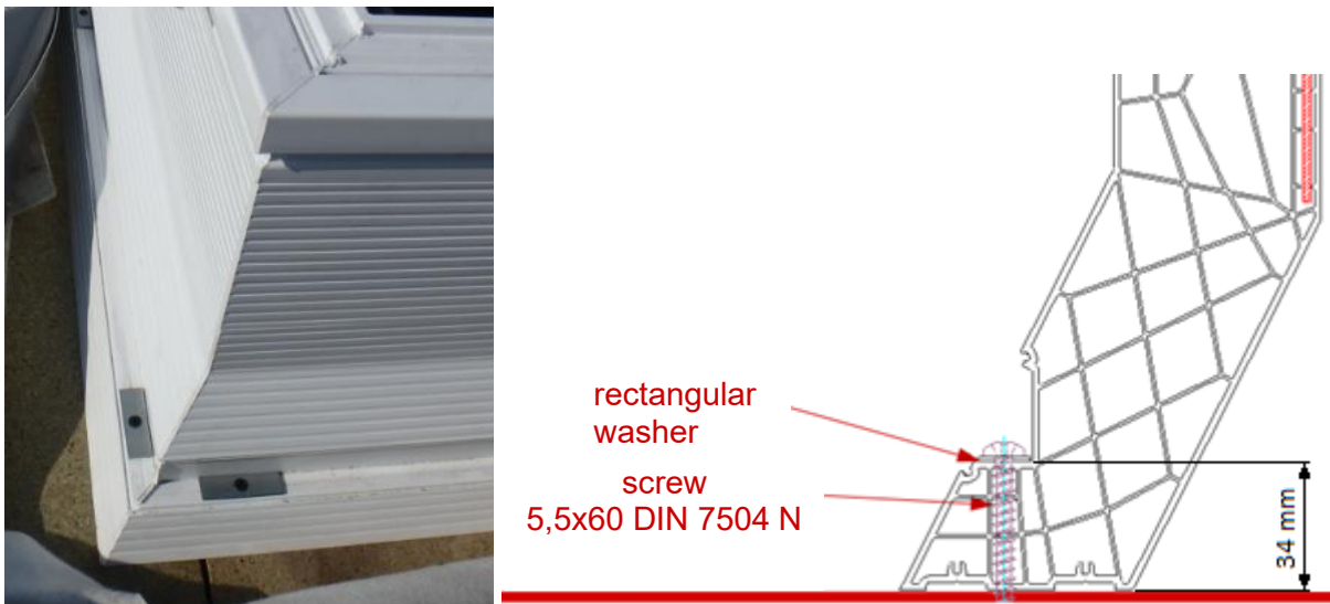
Fig. 16. Fixing the PVC base to the roof
